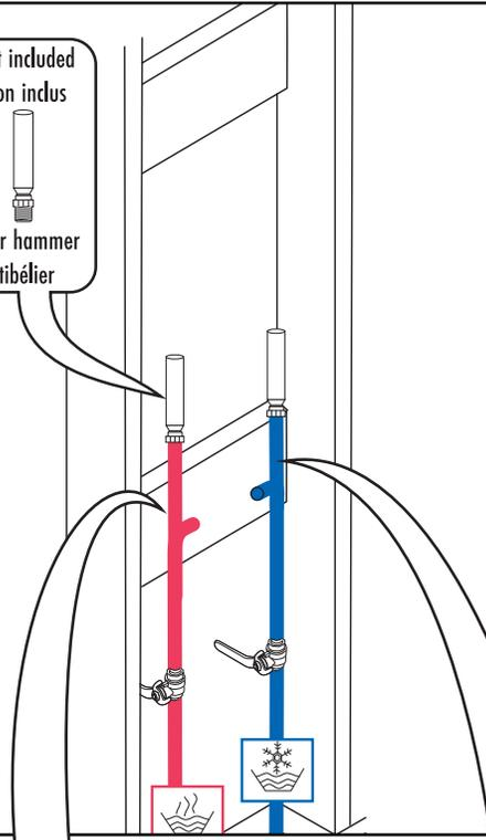
You will need to fix the pipes securely to avoid water hammer.
